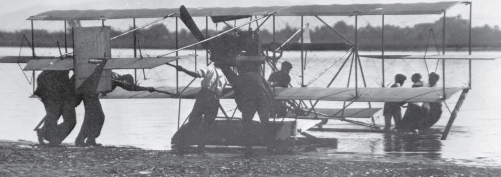
A Curtiss "Hydroaeroplane" is pushed into the water in preparation for flight at North Island in January 1911. On the 26th of the same month this aircraft achieved a notable aviation "first" by being the first aircraft to operate from water. Note that the engine has a pusher propeller and the ailerons are independent of the wings.
